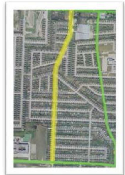
Figure 3-3: Example of Urban Minor Arterial
